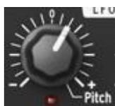
The **Pitch** knob controls the amplitude and polarity of the LFO signal that modulates the oscillator pitch. At the 0 position (12 o'clock) no modulation is sent to the targets. When turned counter-clockwise (below the 0 mark) the **Pitch** knob sends an increasing amount of the inverted LFO signal. When turned clockwise (beyond the 0 mark) the **Pitch** knob sends an increasing amount of the normal LFO signal.
