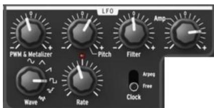
The LFO is a low frequency oscillator. It is the primary modulation source for the MiniBrute's other sections.
