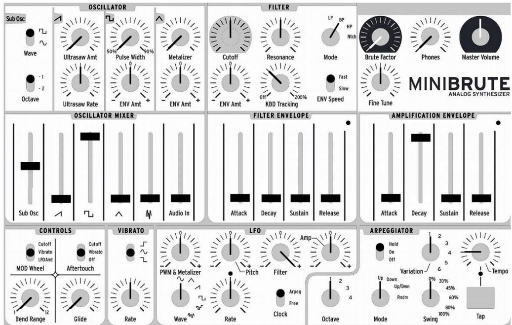
Press the keyboard's lowest C key, then release it: the note auto-repeats continuously, because the arpeggiator is set to **Hold**.
