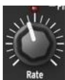
The Rate knob set the LFO oscillation rate, and ranges from very slow rates (0.1Hz) up to quite fast rates (100Hz). The red LED located above the knob blinks in time with the rate. Note that the LFO rate may be superseded by the arpeggiator tempo clock if the **Clock** switch is set to **Arpeg** (see below).
