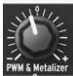
The **PWM & Metalizer** knob controls the amplitude and polarity of the LFO signal that modulates the oscillator pulse wave Pulse Width, and the Metalizer's folding level. At the 0 position (12 o'clock) no modulation is sent to the targets. When turned counter-clockwise (below the 0 mark) the **PWM & Metalizer** knob sends an increasing amount of the inverted LFO signal. When turned clockwise (beyond the 0 mark) the **PWM & Metalizer** knob sends an increasing amount of the normal LFO signal.
