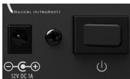
The AC connector receives the MiniBrute's external power supply plug. Only connect the adequate power supply: 12V DC, 1A, center positive.
