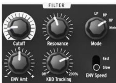
The filter alters the oscillators' timbre via the four response modes described previously (LP, BP, HP & Notch). Its cutoff and resonance can be adjusted manually. The cutoff can also be controlled by the keyboard and modulated by various modulation generators. The MiniBrute filter is based on Nyle Steiner's *Sallen & Key* architecture (designed in the 70s) and offers -12dB/octave slopes in LP and HP modes, and -6dB/octave slopes in BP and Notch modes.
