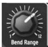
The **Bend Range** knob controls the range of the **Pitch** wheel [4.2.8.2]. With this knob fully counter-clockwise, the Pitch wheel ranges from -1/2 tone (lowest position) up to +1/2 tone. With this knob fully clockwise, the Pitch wheel ranges from -1 octave (lowest position) up to +1 octave.
