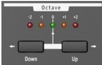
The **Octave** section transposes the MiniBrute keyboard over a wide pitch range. One LED among the five colored LEDs (**-2 red, -1 orange, 0 green, +1 orange, +2 red**) is lit at a time and indicates the transposition octave. The default selection is 0 (green LED), where the leftmost C key corresponds to C2 (130.81Hz) and the rightmost C key corresponds to C4 (523.25Hz).
