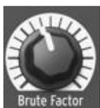
The **Brute Factor** is a special MiniBrute feature inspired by a common patch used on a famous vintage mono-synthesizer that connected the headphone output to the external audio input. The result is a kind of feedback loop that's ideal for raspy and grungy sounds. This patch has been implemented internally to the MiniBrute, and is controlled by the
