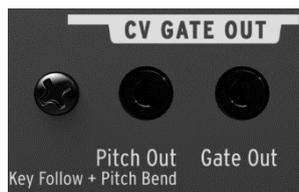
The MiniBrute can also control other analog devices. The **Pitch Out** 1/8" jack provides the CV produced by the MiniBrute keyboard as well as by the Pitch wheel. The keyboard's GATE signal is also available on the **Gate Out** 1/4" jack.
