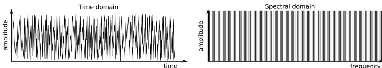
Such signals sound very different from the pitched signals, and are like the sound of wind, a water stream, steam exhaust, rain, waterfall, etc.
