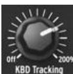
The filter cutoff frequency can also be keyboard-controlled. The **KBD Tracking** knob lets you adjust how the cutoff follows the keyboard. Repeat the exercise described in the Cutoff section, set the **KBD Tracking** knob to 100% (12 o'clock), then play a series of notes on the keyboard. The filter should open more to retain high frequencies as you play higher up on the keyboard.
