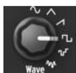
The LFO offers several modulation waveforms, selected by the **Wave** knob: sine, triangle, sawtooth, square, random stepped (also referred to as Sample &
