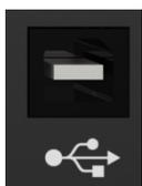
The **USB** outlet interfaces with a personal computer. It can be used for MIDI communication, as well as editing some of the synthesizer internal parameters such as MIDI channel or velocity curves, or updating the arpeggiator firmware, through the MiniBrute Connection software [4.4].
