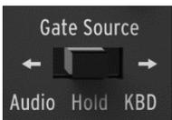
The **Gate Source** switch selects which gate signal triggers the MiniBrute envelopes. The default **KBD** triggers the gate from the keyboard. **Hold** mode forces the envelope to the SUSTAIN stage independently from any other gate source. This mode is very useful for drones, because there is no need to press a key and you can use both hands to tweak the knobs! In **Audio** mode, a gate signal is generated when the signal level at the **AUDIO In** [4.3.5] reaches an internally preset threshold.
