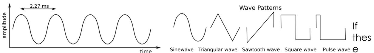
waveforms have the same frequency, then their pitch is equivalent. However, different waveform shapes have different timbres. For example, the sine wave sounds dark and plain, while the sawtooth wave sounds very bright. The square wave sounds a bit like a clarinet and the pulse wave resembles an oboe.
