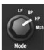
This selects among the four filter modes: **LP** (low-pass), **BP** (band-pass), **HP** (high-pass), and **Notch**. The **LP** mode is the most commonly-used, and provides sounds which are full/fat and round. The **BP** and **HP** modes provide thinner and harsher sounds. When modulated by the LFO, the
