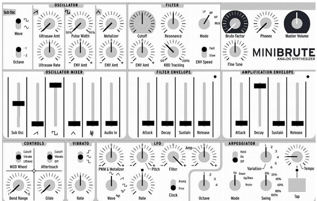
Press and hold a key: you should hear timbre sweeps, a bit like a didgeridoo, at a rhythm indicated by the red LED. Tweak the **Rate** knob to slow down or accelerate this wah-wah effect, and play with the filter's **Resonance** to accentuate it.
