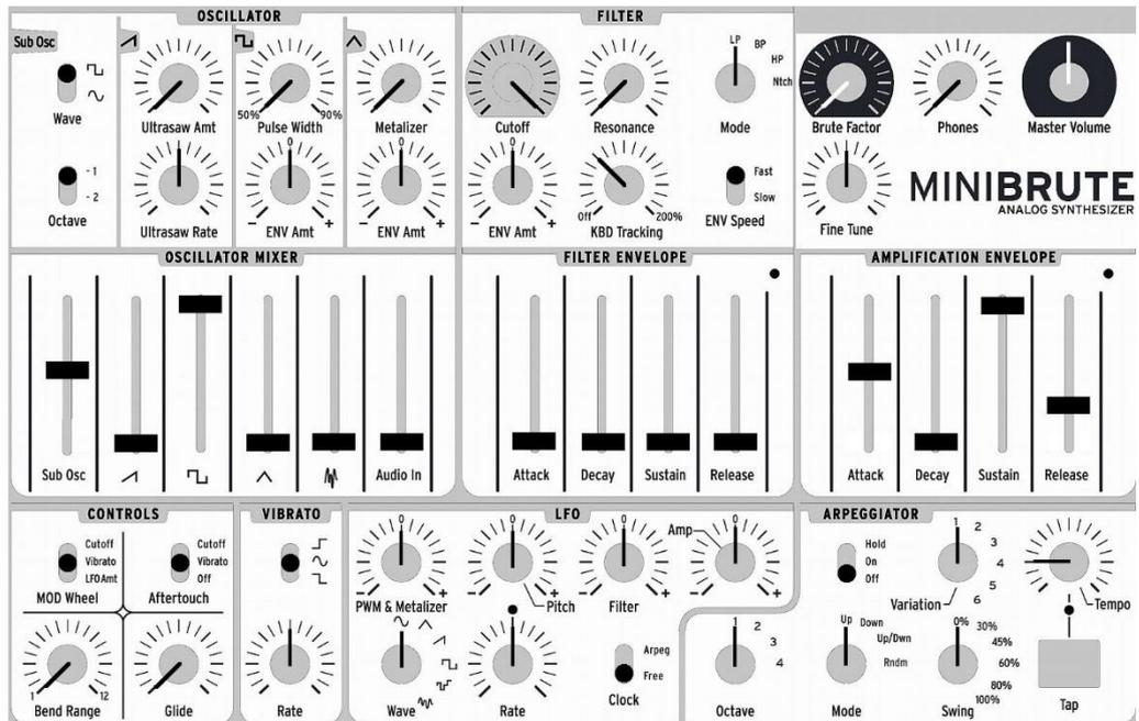
Now set these four envelope sliders all the way down, and raise the **Decay** slider to maximum. Press and hold down a key: the sound appears as soon as you press the key, and slowly fades out to the minimum level. While pressing a key repeatedly, slowly turn down the **Decay** slider: the sound will fade out more rapidly. In the lowest range of the slider, you'll hear short, percussive sounds.
