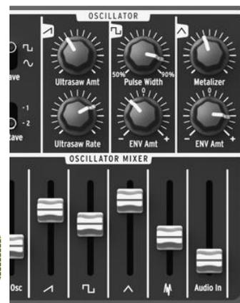
The oscillator delivers three basic waveforms : sawtooth, pulse, and triangle wave. These
